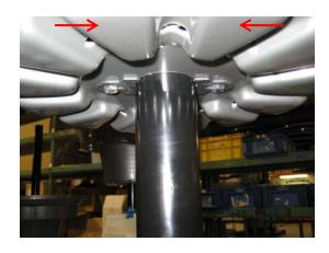
Slide the "Adjustable Clips" into the holes and tighten the two bolts as shown.
